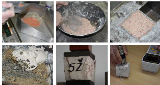
Fig. 2 Conservation mortar models - measuring components, manual mixing of mortar, moulding (top); mortar components, testing compression strength, and colour measuring (bottom) (Photo-documentation of the MoDeCo2000 project)
